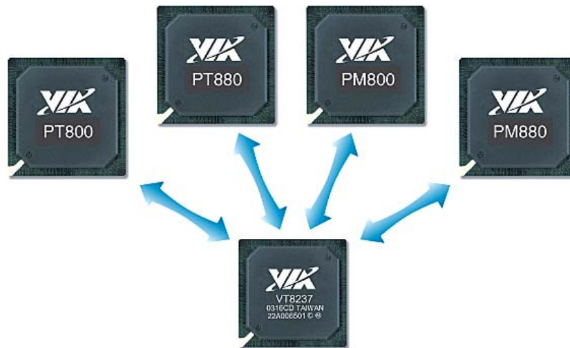
Figure 10: VIA VT8237 Supports Current and Future VIA North Bridges on the Intel Pentium 4 Processor Platform
