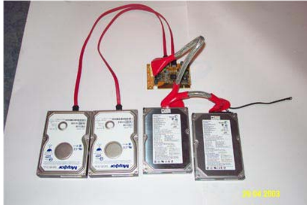
SATA cabling (left) vs. PATA cabling (right)
