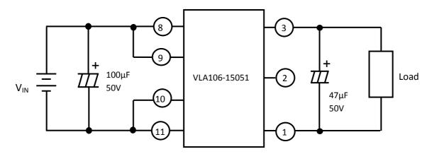
It is used the electrolytic capacitors which has the low impedance.
