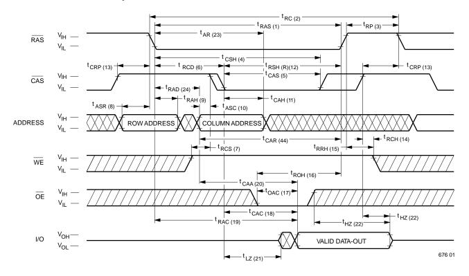
Waveforms of Early Write Cycle
