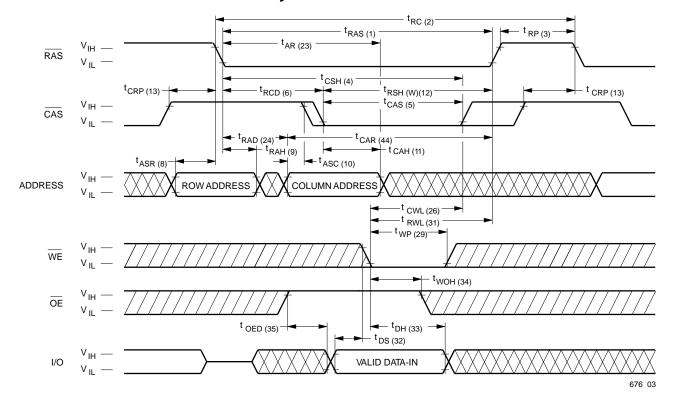
Waveforms of Read-Modify-Write Cycle
