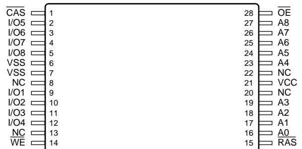
28 Lead TSOP-I PIN CONFIGURATION Top View
