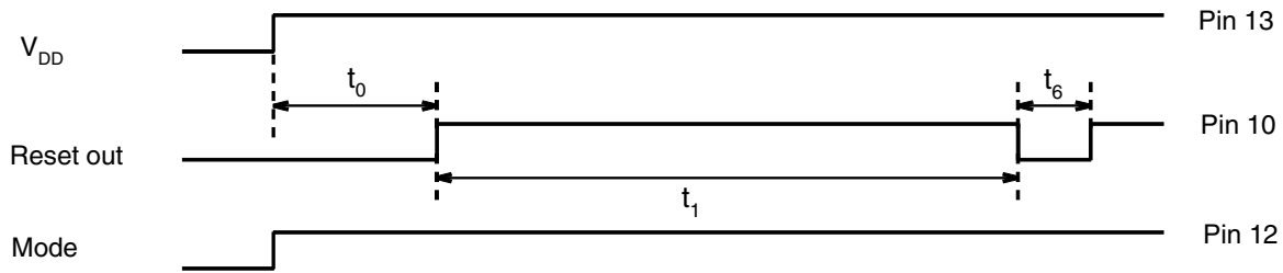
Figure 4. Power-up Reset and Mode Switchover
