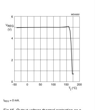
Fig.15 Output voltage thermal protection as a function of the junction temperature.
