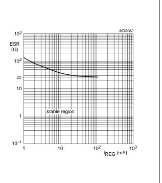
Fig.5 ESR as a function of I<sub>REG</sub> for selecting the value of the output capacitor.
