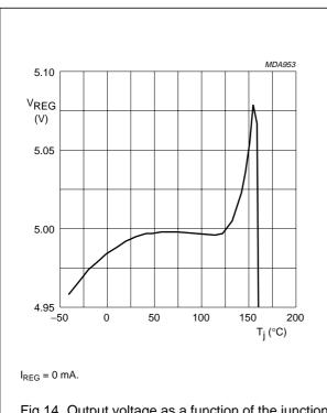
Fig.14 Output voltage as a function of the junction temperature.
