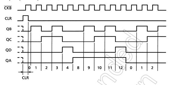
Note: QD connected to  $\overline{\text{CKA}}$
