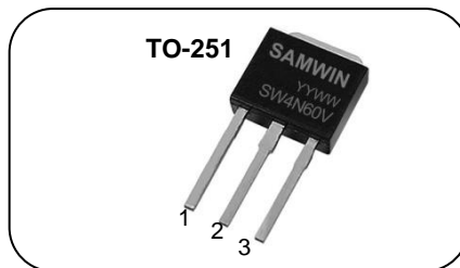
1. Gate 2. Drain 3. Source
