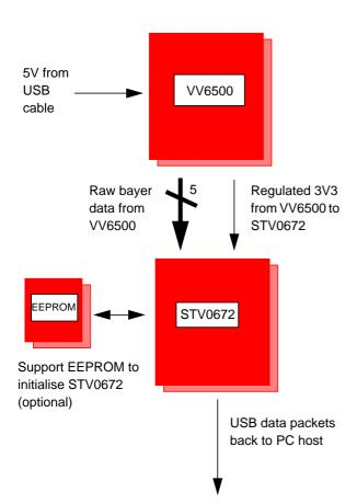
This chipset allows the implementation of a high quality PC camera with a minimum of external components. The support EEPROM is optionally populated if a custom USB enumeration sequence is required.
