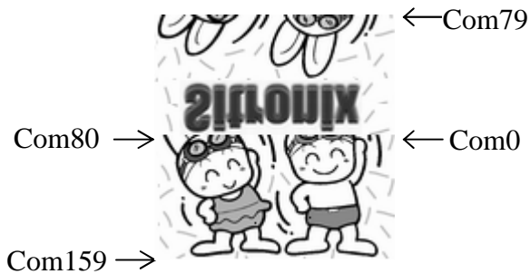
Figure 8.1.1 Common scan direction configuration
