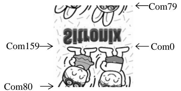
Figure 8.1.1 Common scan direction configuration
