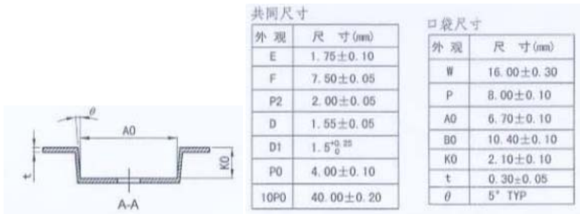
Figure 9 9.9x6 SOP16 Carrier Tape
