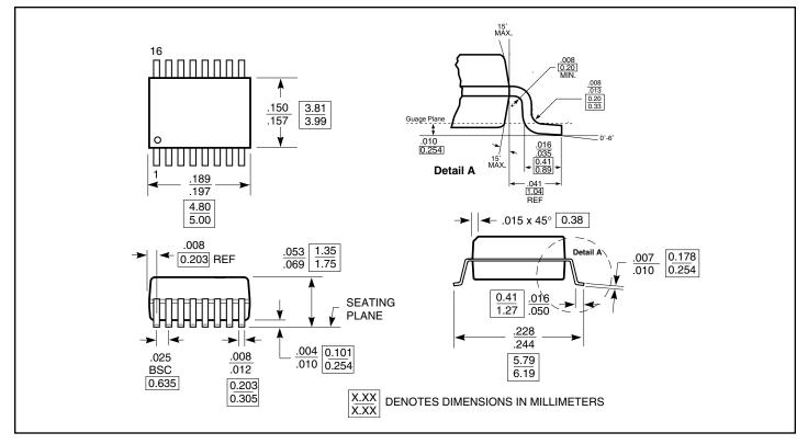
Packaging Mechanical: 16-pin SOIC (S)
