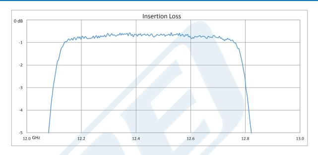
Click the following link (or enter part number in "SEARCH" on website) to obtain additional part information including price, inventory and certifications: 6 Section Bandpass Filter With SMA Female Connectors Operating From 12.2 GHz to 12.7 GHz With a 500 MHz Passband PE87FL1004
