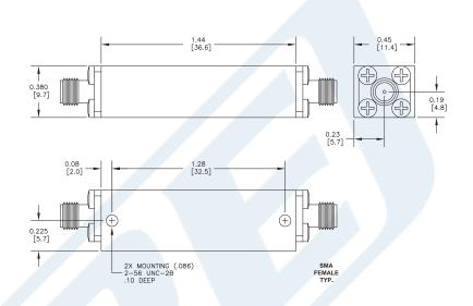
9 Section Bandpass Filter With SMA Female Connectors Operating From 17.7 GHz to 21.2 GHz With a 3.5 GHz Passband from Pasternack Enterprises has same day shipment for domestic and International orders. Our RF, microwave and millimeter wave products maintain a 99% availability and are part of the broadest selection in the industry.
