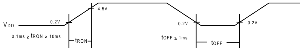
Figure 3. t_{OFF} stipulates the time of power ODD for instantaneous Power supply to or when power supply repeats ON and OFF.
