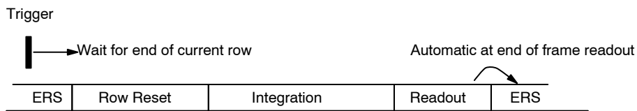
Figure 37. Entering and Leaving a Global Reset Sequence
