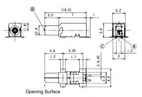
The circuit structure is as described below. Between (A) and (C): Normally closed Between (B) and (C): Normally open
