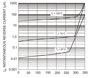
V<sub>R</sub>, INSTANTANEOUS REVERSE VOLTAGE (V) Fig. 3 Typical Reverse Characteristics, per element
