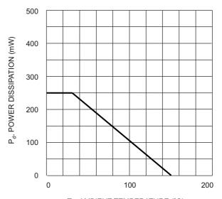
T<sub>A</sub>, AMBIENT TEMPERATURE (°C) Fig. 2 Power Dissipation Derating
