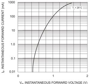
$V_{\rm F}$ , INSTANTANEOUS FORWARD VOLTAGE (V) Fig. 1 Forward Characteristics
