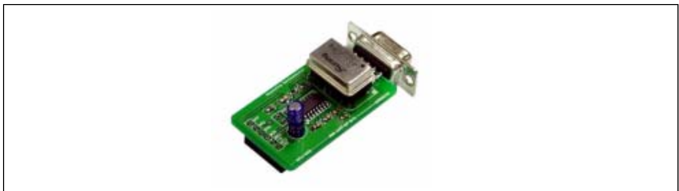
Figure 27-3 MagnaChip supplied ISP Board
