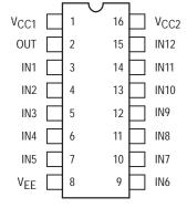
Pin assignment is for Dual–in–Line Package.
