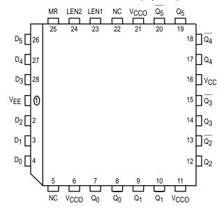
$^{\ast}$  All VCC and VCCO pins are tied together on the die.
