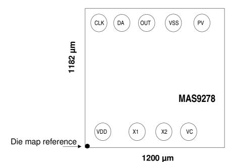
Note 1: MAS9278 pads are round with 80 µm diameter at opening.
