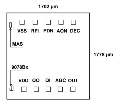
DIE size =  $1.70 \times 1.78 \text{ mm}$ ; PAD size =  $100 \times 100 \mu \text{m}$
