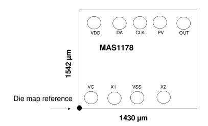
Note 1: MAS1178 pads are round with 80 µm diameter at opening.
