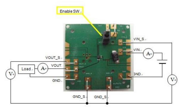
The enable switch has three positions.
