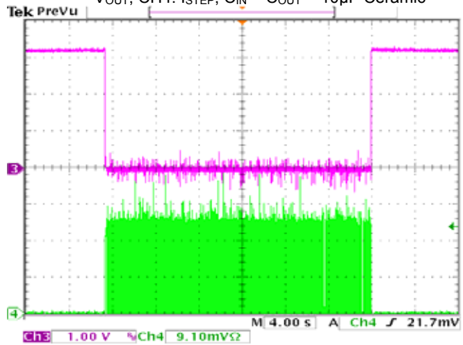
SHORT CIRCUIT AND RECOVERY V_{OUT} , CH4: I_{STEP} , C_{IN} = C_{OUT} = 10\mu\text{F} Ceramic
