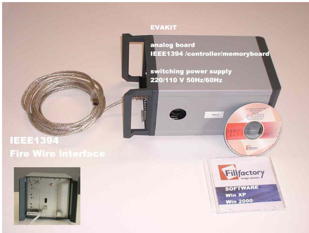
Figure 26: Content of the LUPA-4000 evaluation kit
