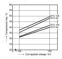
3. Ambient temperature characteristics and coil applied voltage Contact current: 10 A
