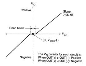
That is, the LB8107M implements a polarity reversing V-type drive with respect to the input signals (from the DSP) referenced to  $V_{REF}1$ .
