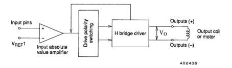
$V_{REF}1$  is supplied from the CD DSP that is powered by the stepped-up voltage (5.0 V) created by the LB8107M. (Normally,  $V_{REF}1$  will be 1/2  $V_{CD}2$ .)
