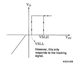
Note that for inputs that are lower than  $V_{REF}1$  this system operates normally regardless of the SLS pin.
