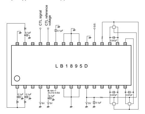
Between power supply and GND, Output and GND, and between Hall inputs:
