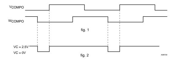
If braking is applied according to the value obtained by OR logic in  $V_{COMPO}$  and  $W_{COMPO}$  together, for example, reverse braking is applied according to the following timing.
