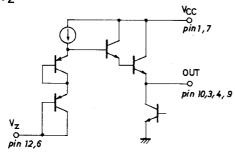
$V_{BE}$  of 2 output NPN transistors is canceled by  $V_{BE}$  of 2 PNP transistors.  $V_o\!\simeq\!V_Z$
