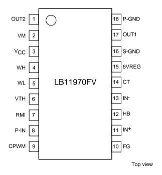
PGND: Motor system GND SGND: Control system GND
