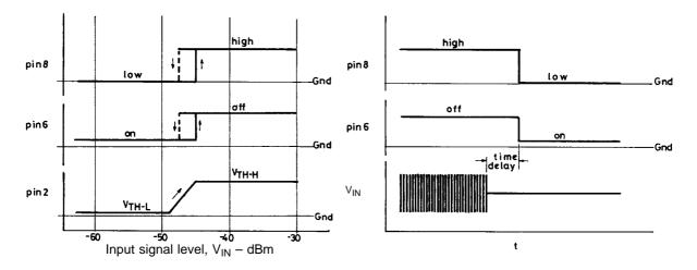
As shown above, when input level is raised and the pin 2 voltage reaches the  $V_{TH-H}$  level of the comparator, pins 6 and 8 turn over. ( $V_{IN} = -45$  dBm).
