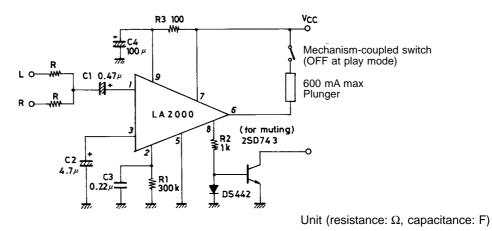
Pin 4 is unconnected but is not be used for GND or an interconnection terminal.
