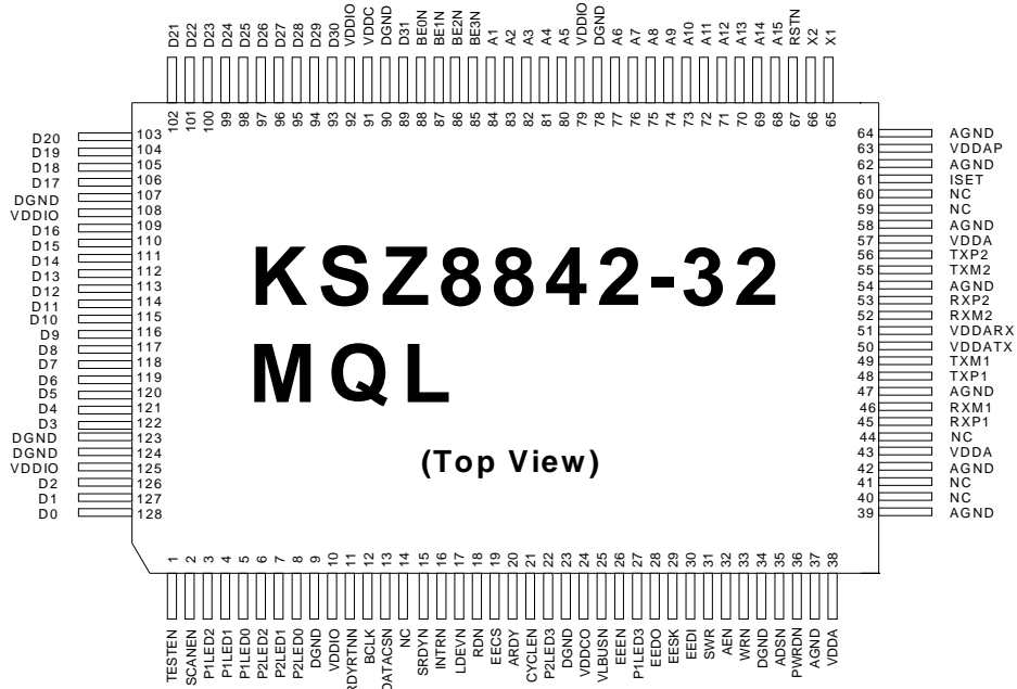
Figure 5. Standard – KSZ8842-32 MQL 128-Pin PQFP (Top View)
