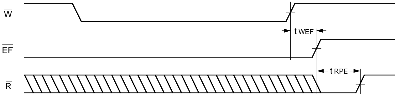
Figure 7. Minimum Timing for an Empty Flag Coincident Read Pulse
