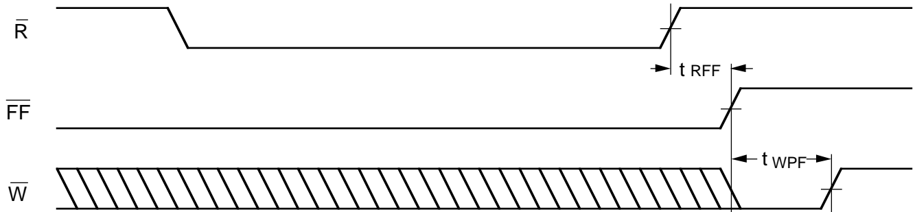
Figure 8. Minimum Timing for a Full Flag Coincident Write Pulse
