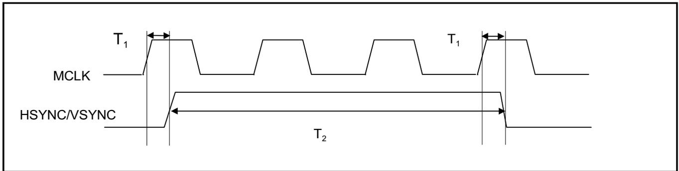
$T_1$  : MCLK rising to HSYNC/VSYNC valid maximum time : 18ns [output load: 60pF]
