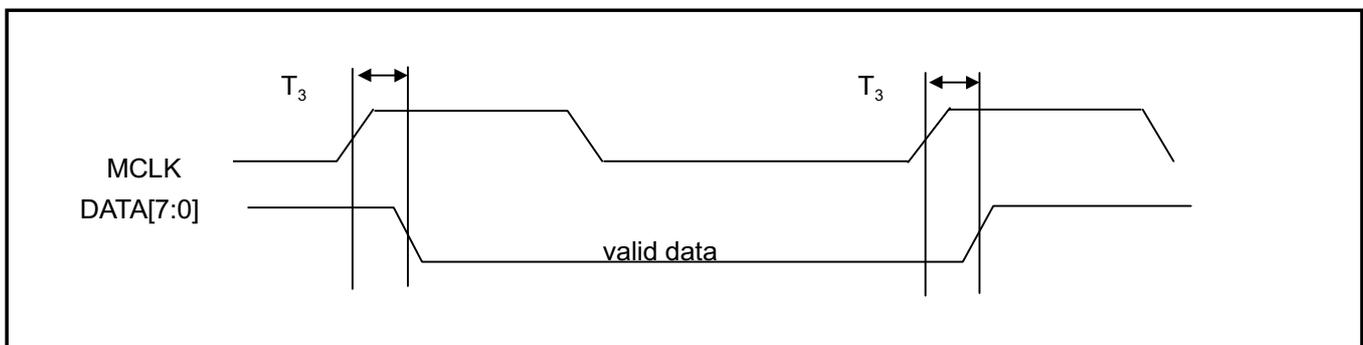
$T_3$  : MCLK rising to DATA valid maximum time : 18ns [output load: 60pF]
