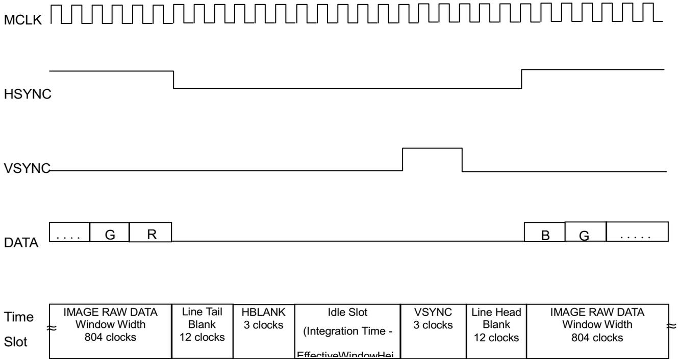
$$\text{Integration Time} > \text{EffectiveWindowHeight} * \text{Scale}$$
