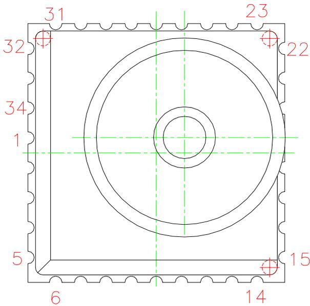
Pin9~16, Pin19~20, Pin33~41 : No Connection
