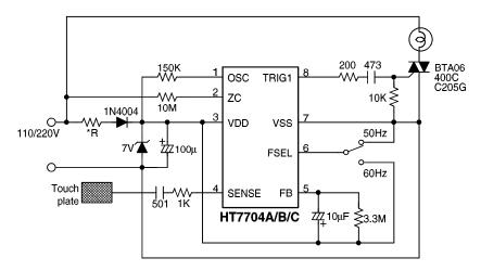
$^*$  Note:1) R=22K $\Omega$ /2W when the AC power supply is 110V. R=43K $\Omega$ /2W when the AC power supply is 220V.
