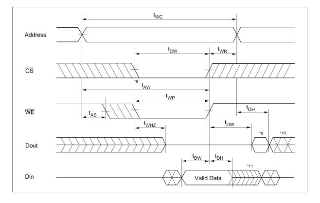
Write Timing Waveform (2) (OE Low Fixed)
