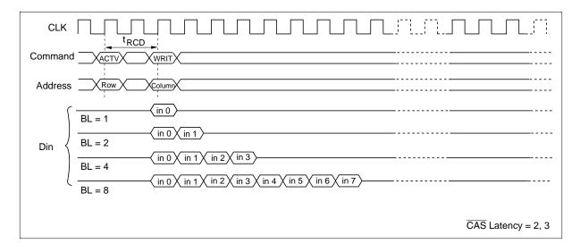
**2. Single write:** A single write operation is enabled by setting OPCODE (A9, A8) to (1, 0). In a single write operation, data is only written to the column address and the bank select address (BA0/BA1) specified by the write command set cycle without regard to the burst length setting. (The latency of data input is 0 clock).
