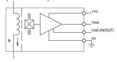
(\*) should be connected to 0V of Power Supply for better dv/dt immunity. Arrow indicates positive current direction.
