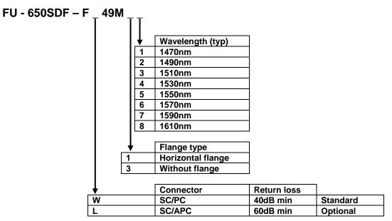
1.55  $\mu\text{m}$  DFB-LD MODULE WITH SINGLEMODE FIBER PIGTAIL
