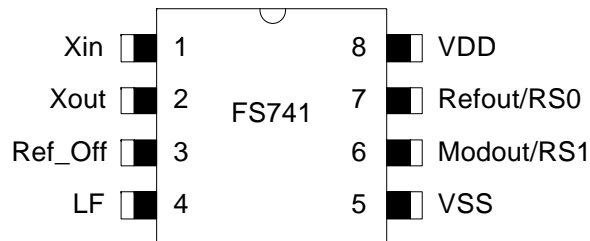
Figure 2. FS741, SOIC Package Pin Assignment
