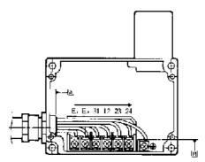
Tighten each wired terminal clockwise to a torque of 0.59 to 0.78  $\mbox{N}\cdot\mbox{m}.$
