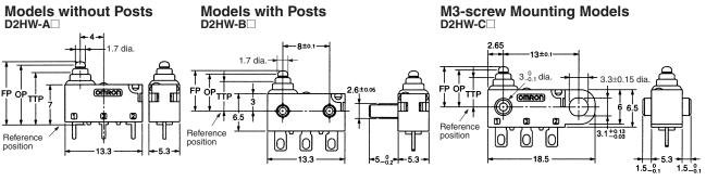
Mounting Hole Dimensions (Reference) Mounting Hole Dimensions (Reference)
