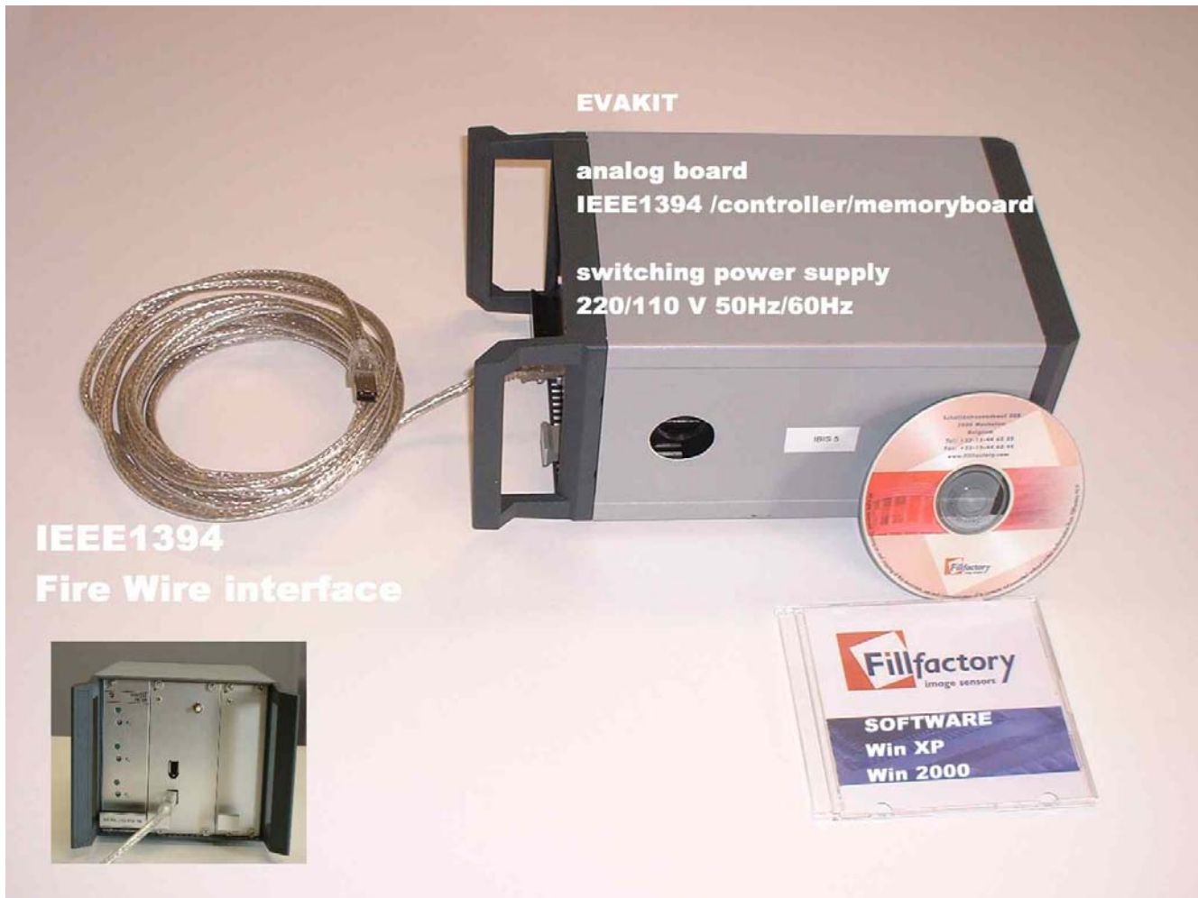
Figure 27. Contents of LUPA 4000 Evaluation Kit
