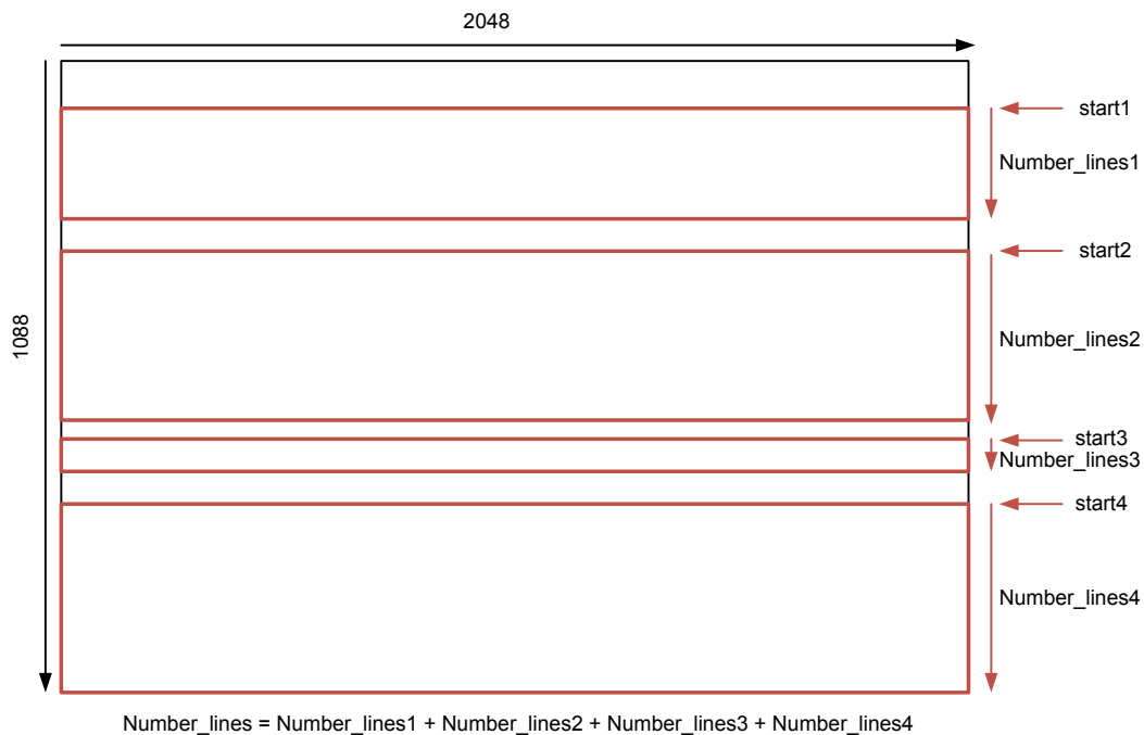
FIGURE 39: EXAMPLE OF 4 MULTIPLE FRAMES READ-OUT
