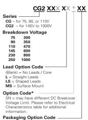
(Blank) = No Leads / Core, Bulk Bag - 400 pcs L(Blank) = Straight Lead, Tray - 50 pcs LTR = Straight Lead, Trape & Reel per EIA RS-296-E - 500 per reel LTE = Straight Lead, Tape & Reel per IEC 60286-1 - 500 per reel LS(Blank) = Shaped Lead (see LS dimensions), Tape & Reel - 500 per reel
