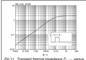
Fig.11. Transient thermal impedance  $Z_{th j\text{-mb}}$ , versus pulse width  $t_n$ .
