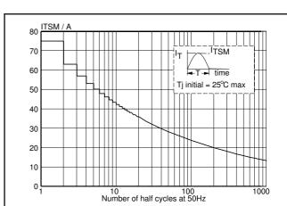
Fig.4. Maximum permissible non-repetitive peak on-state current  $I_{TSM}$ , versus number of cycles, for sinusoidal currents, f = 50 Hz.
