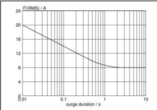
Fig.5. Maximum permissible repetitive rms on-state current  $I_{T(RMS)}$ , versus surge duration, for sinusoidal currents, f = 50 Hz;  $T_{mb} \le 111$  °C.
