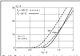
Fig.10. Typical and maximum on-state characteristic.
