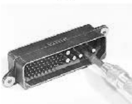
Extracting Coaxial & #12 Contacts
