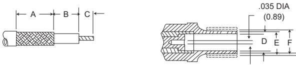
50 Ohm Contact (RG-196U) (assembly steps 1, 2, 3, 4, 5 & 8)
