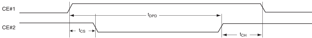
Figure 32. Deep Power-down Timing
